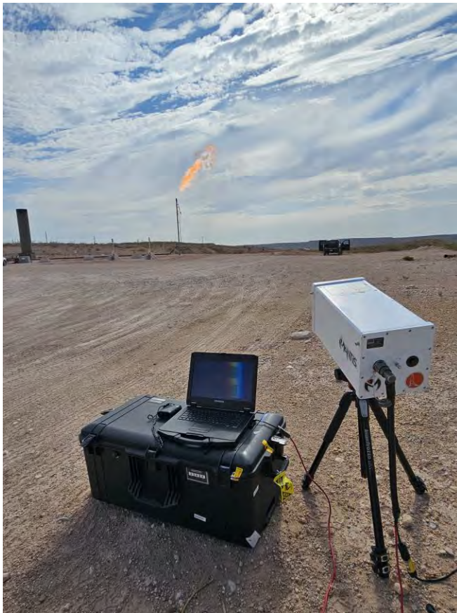
Figure 1: Mantis deployed during API field survey in Barnett region.
